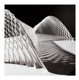
Taking inspiration from Japanese tea bowls and fish scales, architect <u>Kengo Kuma</u>'s metal screen installation is intended to be an indoor and an outdoor space at once. While the structure's thin metal shell looks like it offers little protection from the elements, it is actually lined with a waterproof membrane.
